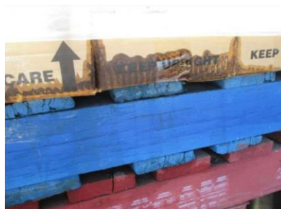
Example: Poorly stacked pallet of liquids. Placing a board or sheet at the base of a pallet will assist with an even weight distribution. The bottles of liquid in these cartons have leaked due to pallet board unevenness and uneven weight distribution.
