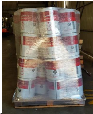
Example: Poorly stacked pallet. Pallet is stacked with spaces between the tins and wrapped too tight resulting in the tins collapsing at the top and all coming together.
