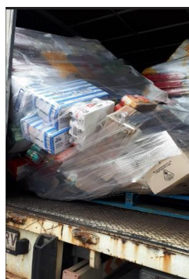
Example: Over height and poorly packed pallet
