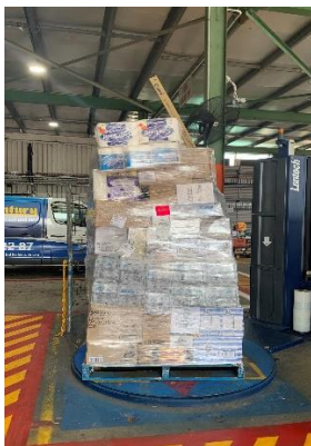
Example: Over height and poorly packed pallet
