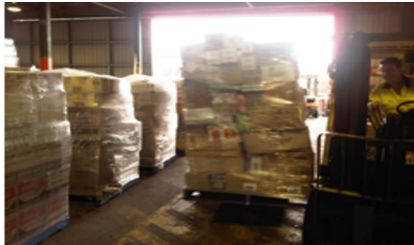
Example: Poorly packed pallet
